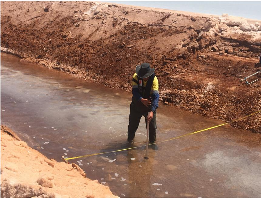
Water Velocity Measurement in Hypersaline Discharge
